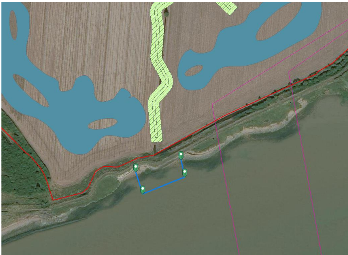
Plate 2: Proposed amendments to the DCO Order Limits to provide the 50mx20-35m working space for the construction of the sluice structure. Approximate amendments to Order Limits to incorporate flood defence also highlighted.
